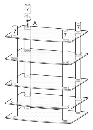
Screw cylinders (7) onto long rods (A). Note that cylinders (7) will fit snuggly inside the decorative rings placed in the previous step.
